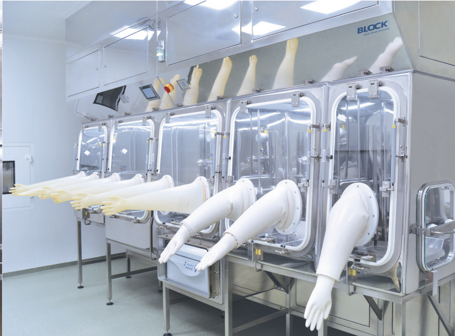
Isolator for working with mammalian cells and tissues, Biocetix S.A., Poland
