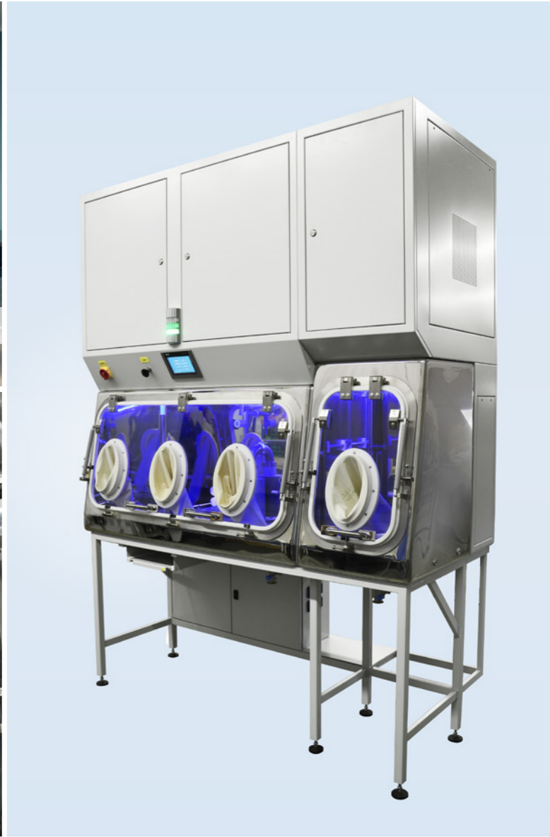
Isolator for work with cytostatics, Rafarma, Russia
