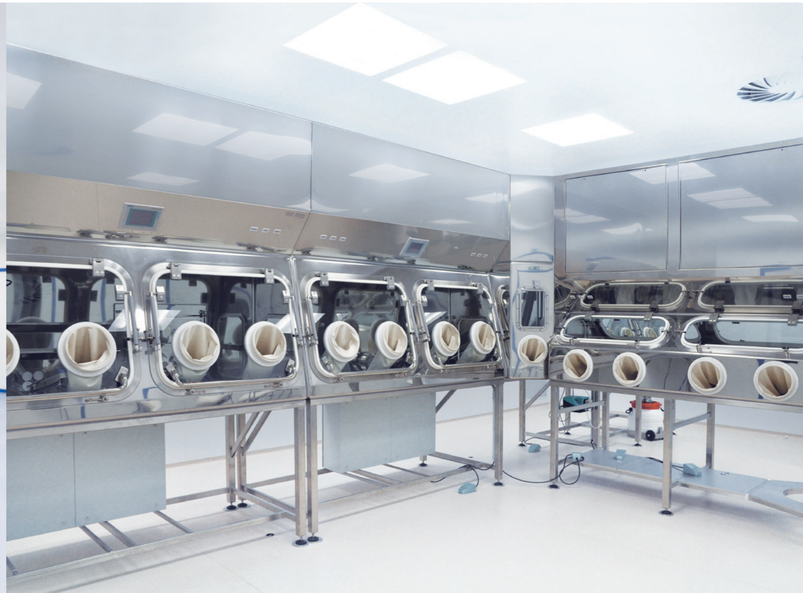
Isolator for product protection - for working with human tissues in a sterile environment, National Tissue Centre Inc., Czechia
