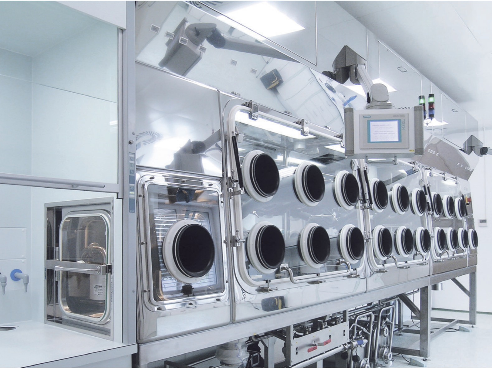
Isolator for working with hazardous materials, Zentiva Group a.s., Czechia
