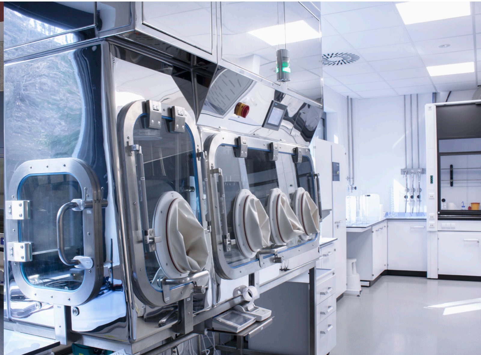
Negative pressure isolator for protect of the personal, processed material API, light sensitive, humidity sensitive Synthon, s.r.o., Czechia
