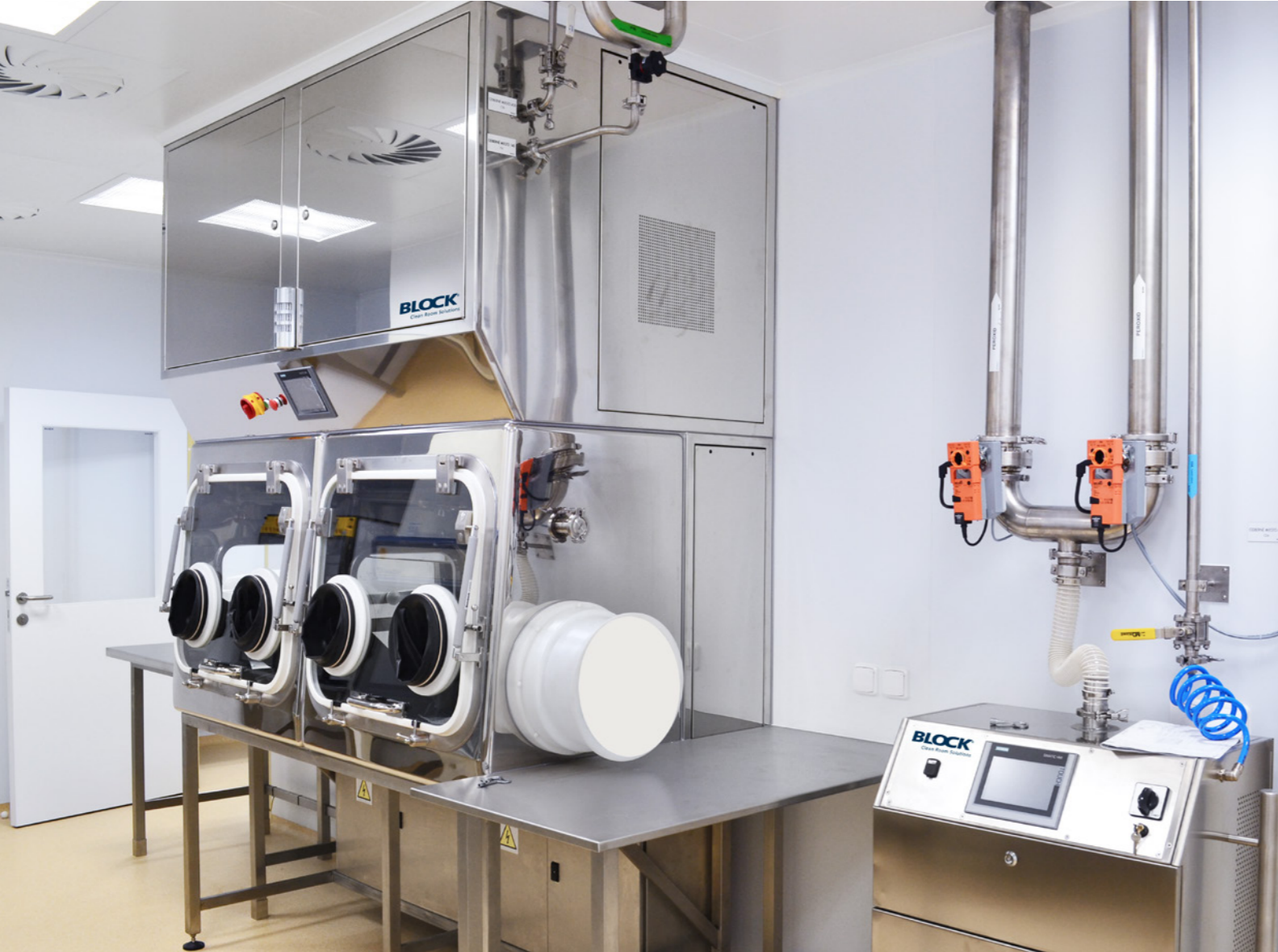
Isolator for work with hazardous materials aseptically; Slovak Academy of Sciences; Slovakia
