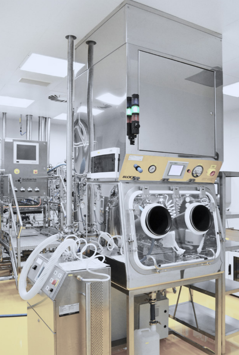
Isolator for handling viruses and infectious substances, Biotechnological Hall (Bioveta Tech Hall), Bioveta a.s., Czechia
