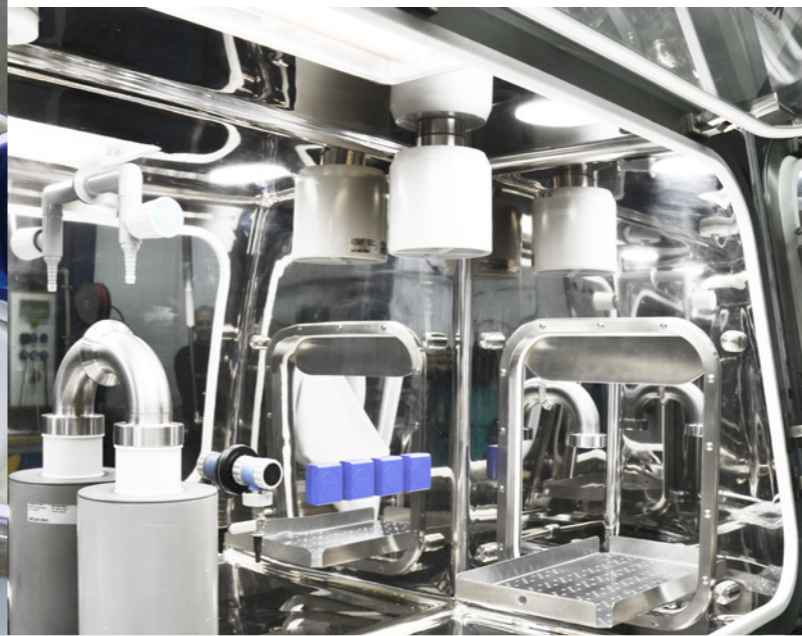
Isolator for work with cytostatics, Rafarma, Russia
