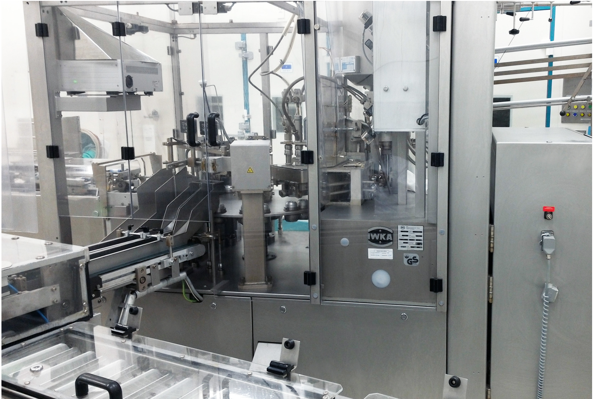
RABS (Restricted Access Barrier System) | Zentiva, k.s. | Czech Republic
