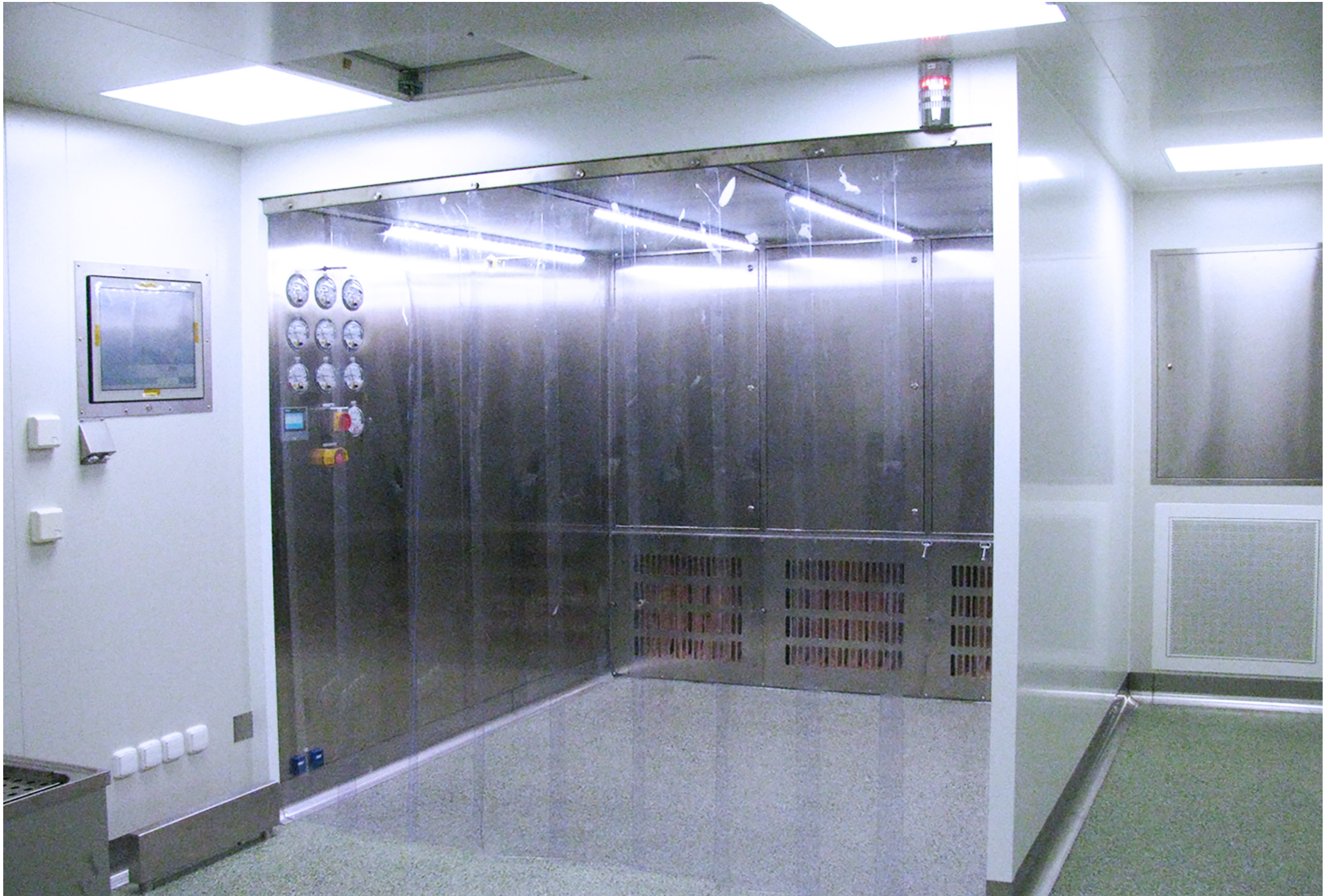
Weighing box for weighing loose materials and consists of a working and an installation space | Teva Czech Industries s.r.o., Opava | Czech Republic
