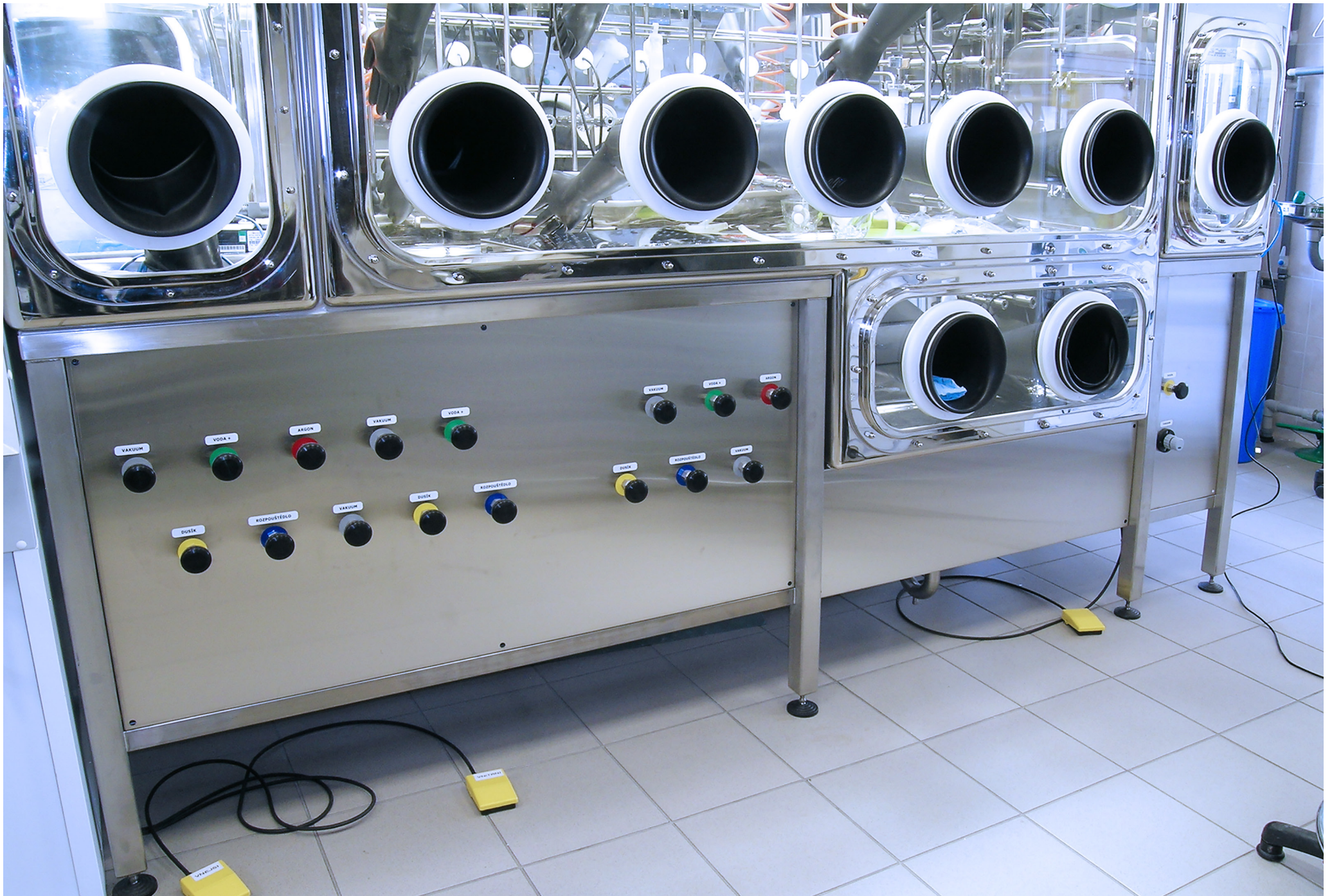
Intended for the research into HPP synthesis and isolation of semi-finished products or their purification | IVAX Pharmaceutical s.r.o., Opava | Czech Republic
