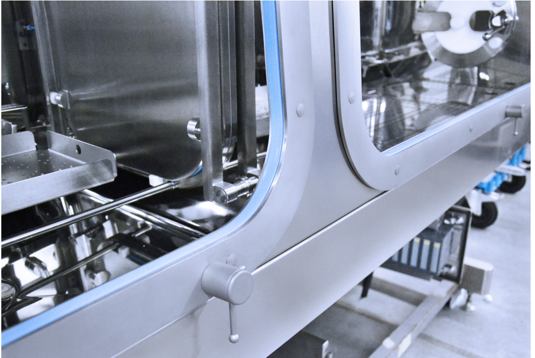
Isolator for work with toxic substances
