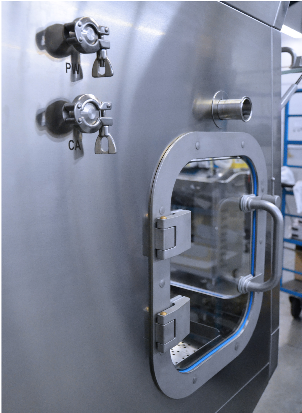
Isolator for work with toxic substances
