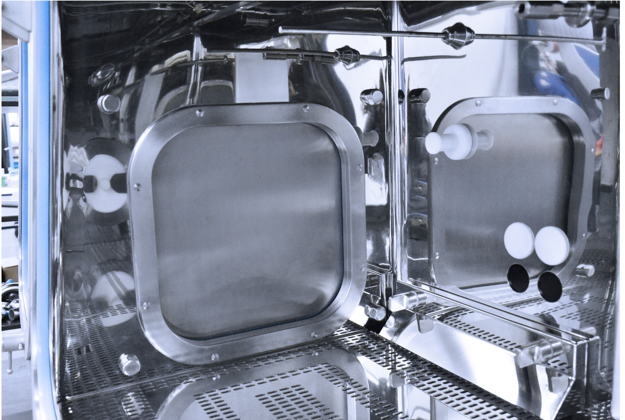
Isolator for work with toxic substances
