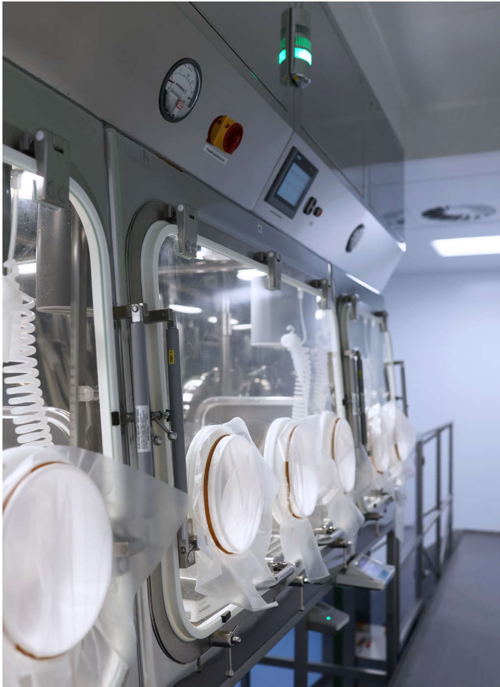
Isolator technology for weighing API hormones | Veropharm - Abbott | Russia
